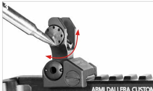
To set the rear sight to the point of impact **turn anti-clockwise to move left** the sight and **turn clockwise to move right** the sight.
