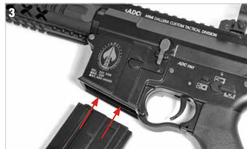
Insert the magazine in the receiver **as shown.**
