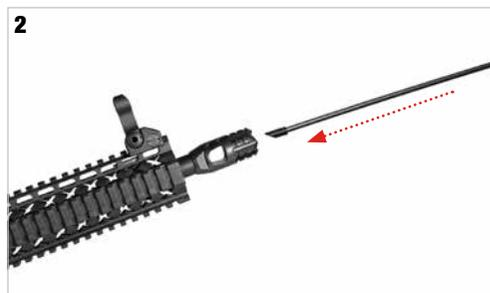
In case of **defective BB's jammed** inside the barrel or in the Hop Up chamber, **immediatly stop firing**, adjust the Hop Up to minimum, **remove the magazine** and use the **unjamming rod** to push the clogged BB outside the Hop Up chamber feeding hole.
