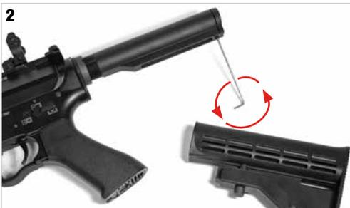
**2** Open the cover of the buffer tube using a hex wrench.
