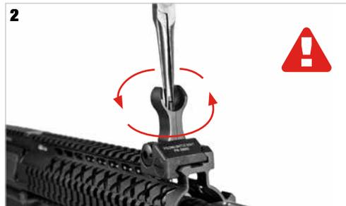
To set the front sight to the point of impact **turn anti-clockwise to move up** the sight and **turn clockwise to move down** the sight.
