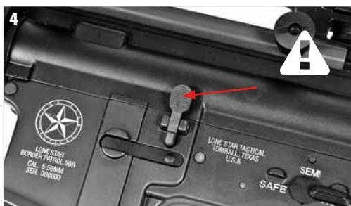
Press **the upper part** of the bolt catch lever **to release the dummy bolt**.
