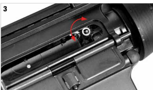
After **each use** set the Hop Up to zero to **release the stress on the Hop Up packing**.
