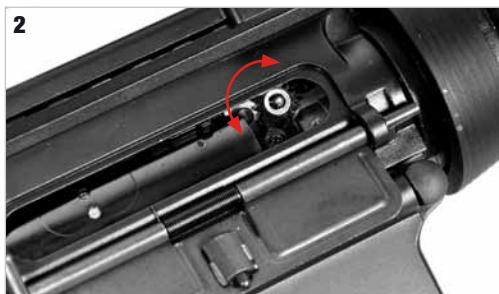
**To adjust the Hop Up** **turn the gear clockwise** to increase the effect and **counter-clockwise** to decrease it.
