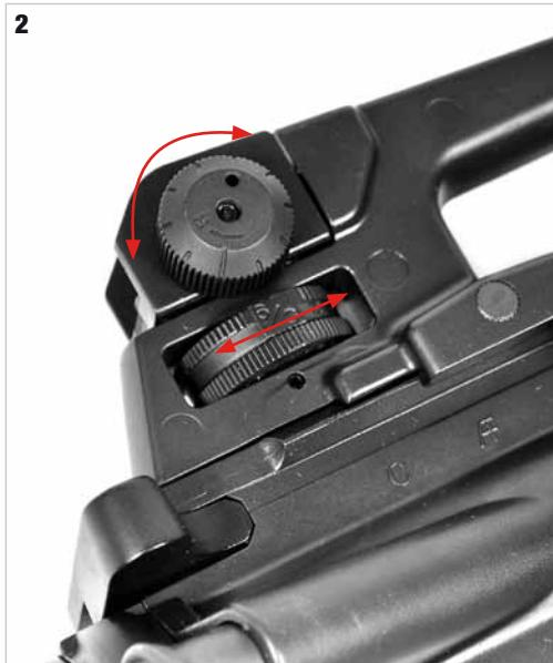
To set the rear sight to the point of impact **turn anti-clockwise to move left** the sight and **turn clockwise to move right** the sight. For rear sight **up or down adjustment** turn the wheel **clockwise to raise** the point of impact and turn **anti-clockwise to lower it**.
