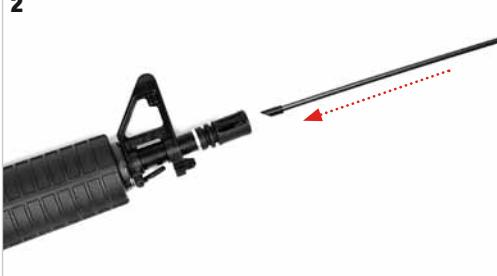
In case of **defective BB's jammed** inside the barrel or in the Hop Up chamber, **immediately stop firing**, adjust the Hop Up to minimum, **remove the magazine** and **use the unjamming rod** to push the clogged BB outside the Hop Up chamber feeding hole.
