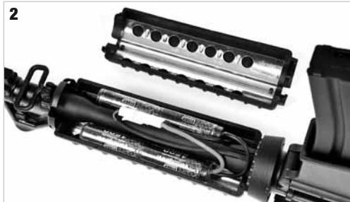
**Insert the battery in the handguard as shown and connect the connectors. Store the connectors over the barrel as shown.**
