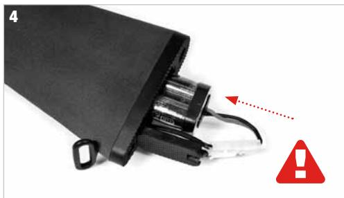
**Insert the battery into the stock, connect the connectors and close the cover.**
