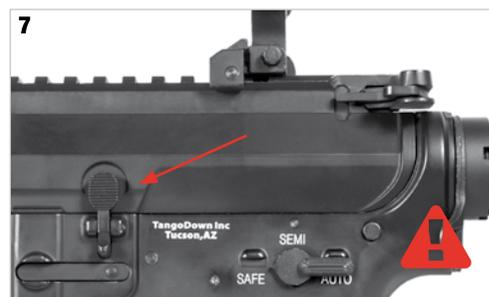
Press **the upper part** of the bolt catch lever **to release the dummy bolt**.
