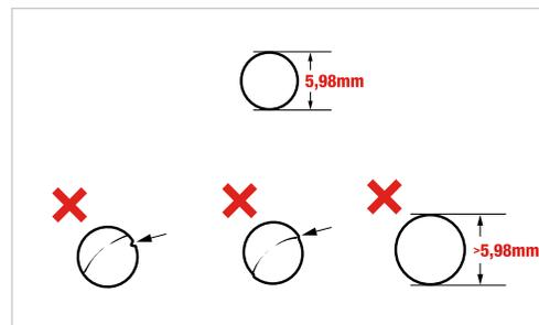
**Use exclusively new BB pellets is a must. Do not use any BB pellet which is not completed, any broken BB pellet and any BB pellet which actual diameter exceeds 5,98mm.**
