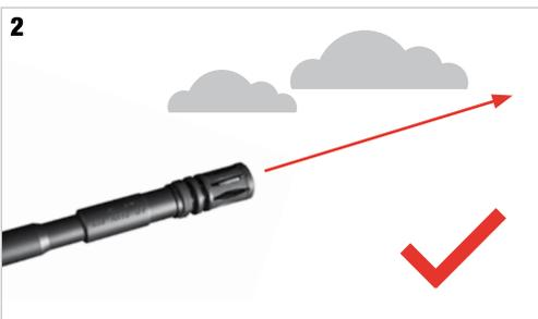
Direct the muzzle **to a safe direction** and shoot two-three **blank firings** to unload the main spring.
