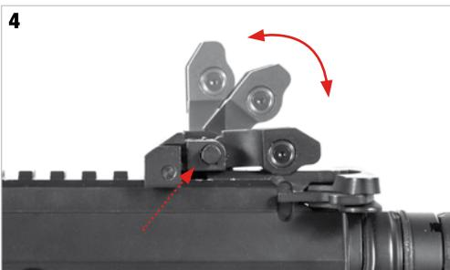
The **TangoDown ECR** is equipped with **folding sights** to allow the use of **additional aiming devices** (Red Dots, Rifle Scopes, Night Vision Devices, etc.).
