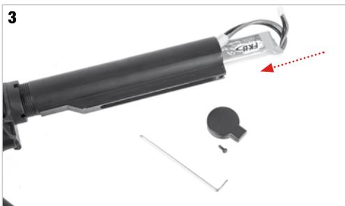
**3** Insert the battery in the buffer tube as shown and connect the connectors. Close the cover and reposition the stock on buffer tube.
