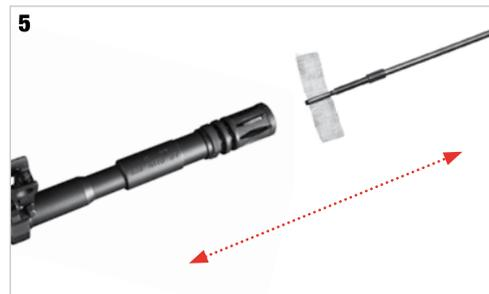
After **each use** always clean **the barrel** using the **cleaning rod provided** and a small piece of fabric, **soaked in silicone oil**.
