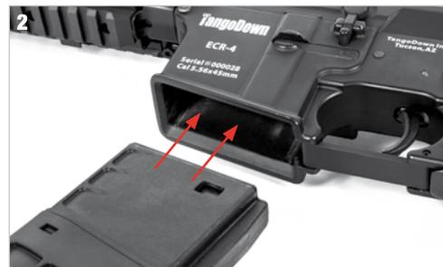
**2** Insert the magazine in the receiver as shown.
