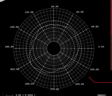
Three-dimensional scan of Xtreme Precision® BB surface (Magnified 1000 times). The test report shows the astonishing average roundness value of 1,088µm
